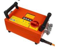
Of course, I am noise emission suppressed. This is important to prevent any disturbances with computer, radio- and television systems. You can also start and operate me via a fault current protective switch with a rate current of 30mA because my filter is producing a low leakage current.
